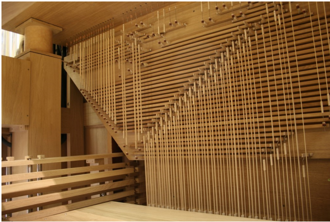
Mechanical/Tracker action in large tracker organs can be very complicated!
