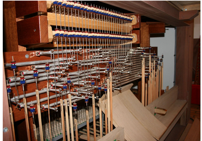
Looking behind the mechanical/tracker action
